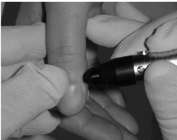
Fig. 1. Measurement of electric current with point electrode at the corner of the fingernail (point n. RH-1, see Table 1).
