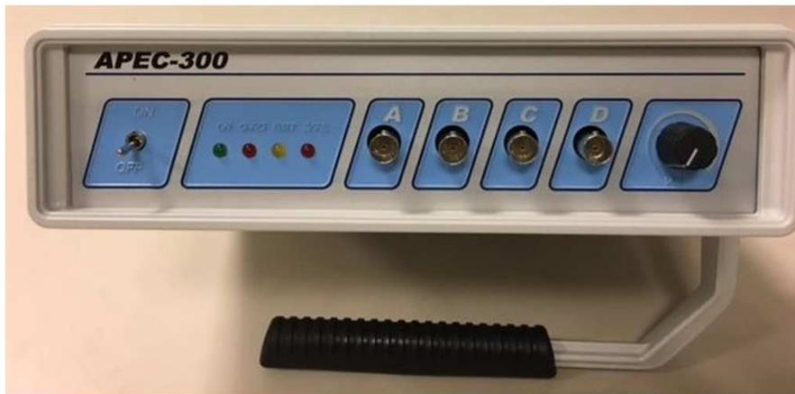
The possibility of a more “at hand” measure, by APEC 300, of *potential variations* of about ten nV (nanoVolt), together with analyzing the spectrum in ultra-low frequency region, could provide some interesting and reliable results in a less demanding way.
