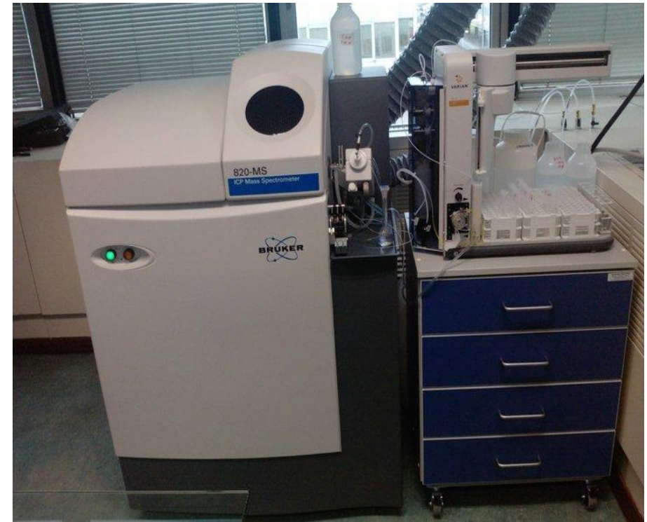
ICP-MS analysis of the solutions is the 820MS of Bruker Daltonics, also equipped with autosampler SPS3 Varian
