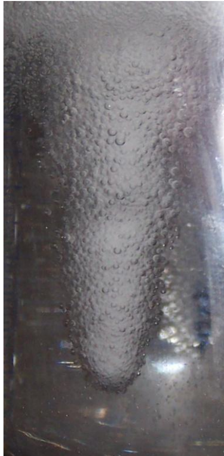
Hydrogen generation at cathode
